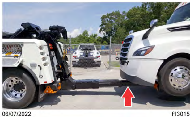
Fig 226, Retracting the Recovery Boom
