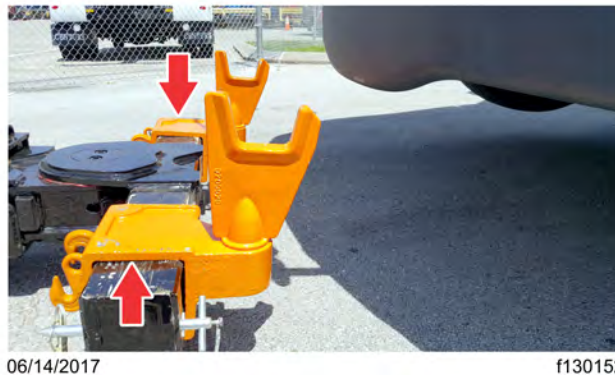
Fig 224, Lift Adaptors Installed on the Crossbar
