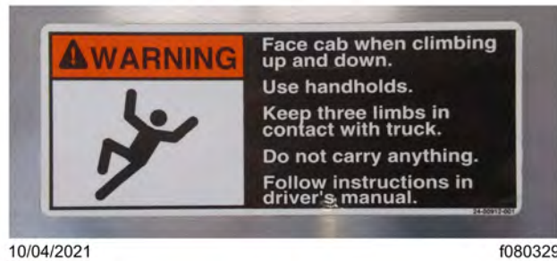
Fig 20, Cab Access Warning Label
