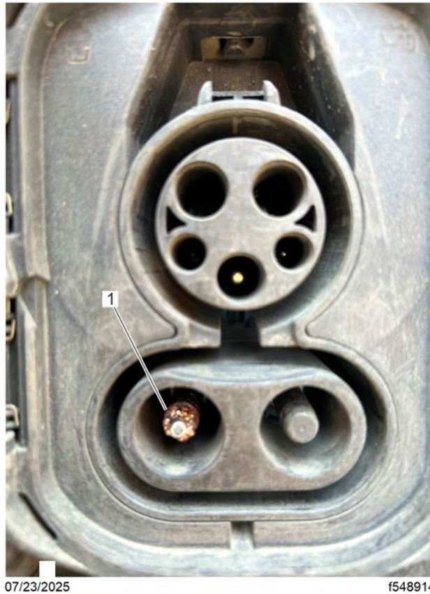
Fig 134, Damaged Charge Port Inlet
