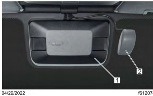
Fig 77, Multipurpose Camera 2 and Bendix Camera Brackets
