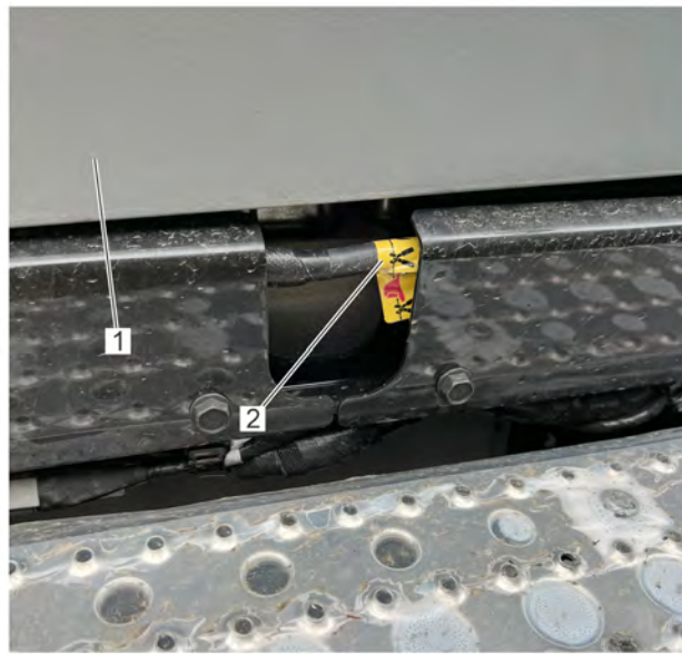
Fig 281, Emergency Responder Cable Cut Point
