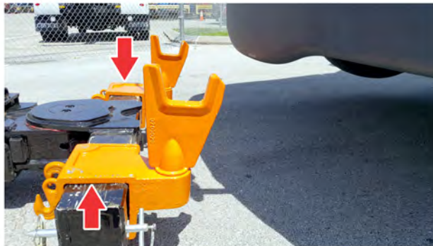
Fig 297, Lift Adaptors Installed on the Crossbar
