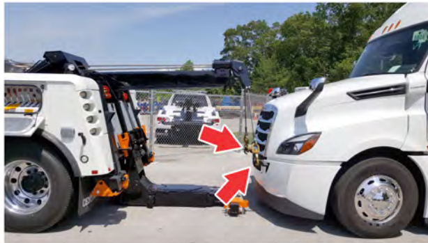
Fig 295, Tow Cables Connected to the Tow Loops
