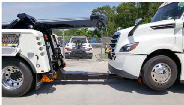
Fig 300, Stinger with Lift Adaptors Under the Axle (tow truck shown)
