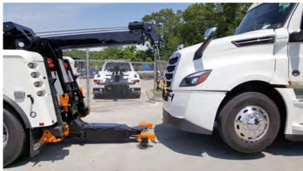
Fig 296, Moving the Stinger and Crossbar Under the Bumper
