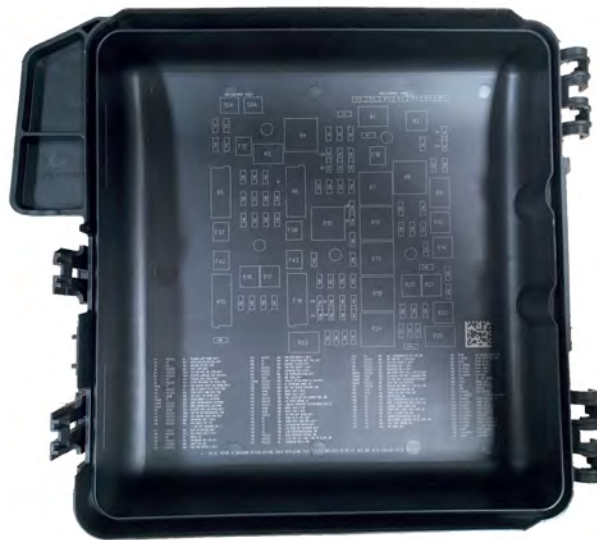
Fig 128, EVDM Inside Cover Map of Fuses and Relays
