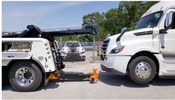
Fig 298, Backing the Tow Truck with Lift Adaptors on the Crossbar
