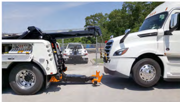
Fig 430, Backing the Tow Truck with Lift Adaptors on the Crossbar
