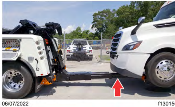
Fig 433, Retracting the Recovery Boom
