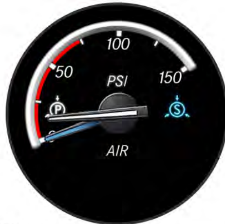
Fig 98, Analog Combined Application Air Pressure Gauge - ICUC
