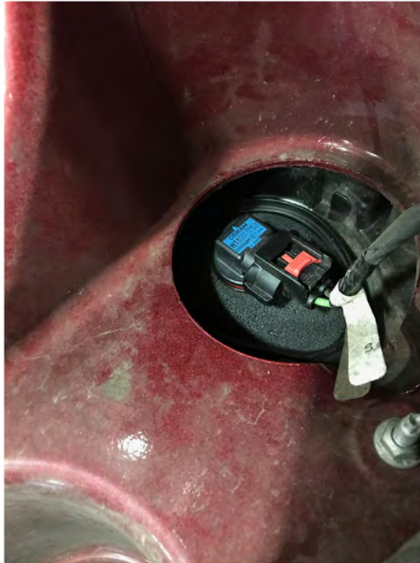
Fig 407, Correct Halogen Headlamp Installation With Foam Grommet
