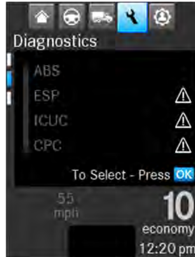
Fig 303, Electronic Control Unite (ECU) List in the ICUC
