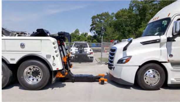
Fig 426, Positioning the Stinger Assembly
