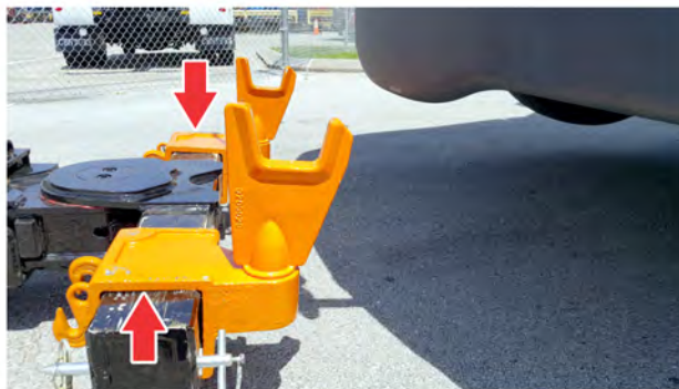
Fig 429, Lift Adaptors Installed on the Crossbar
