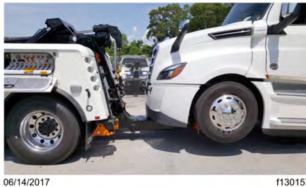
Fig 434, Final Towing Position
