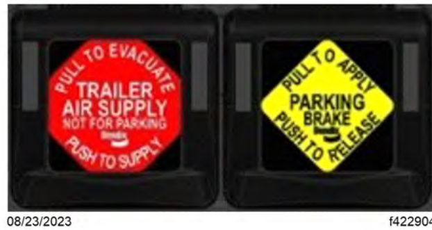
Fig 201, Tractor Parking Brake Released and Trailer Spring Brakes Released
