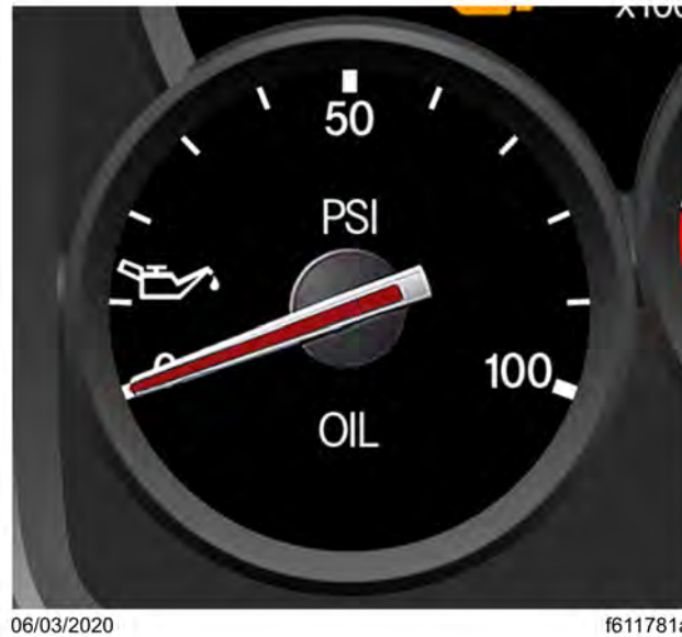
Fig 74, Analog Engine Oil Pressure Gauge - ICUC
