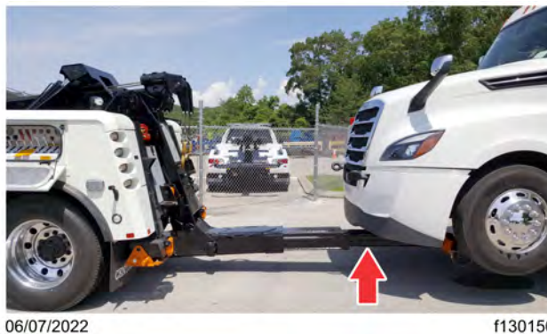
Fig 339, Retracting the Recovery Boom
