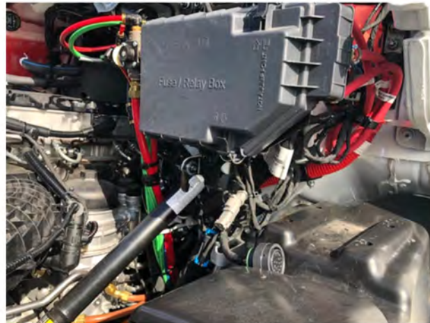
Fig 171, Power Distribution Module (PDM) in Engine Compartment
