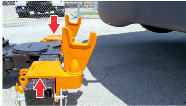
Fig 335, Lift Adaptors Installed on the Crossbar
