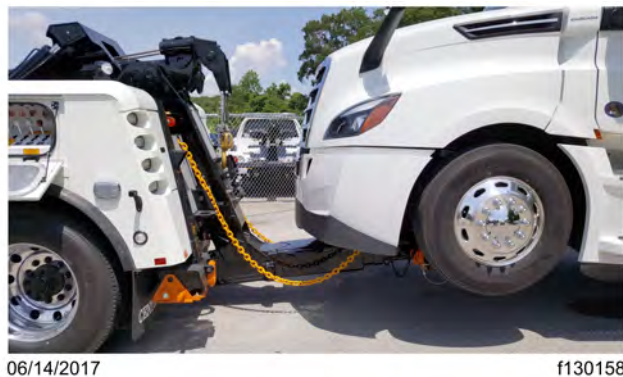
Fig 341, Safety Chains Connected on the Towed Vehicle
