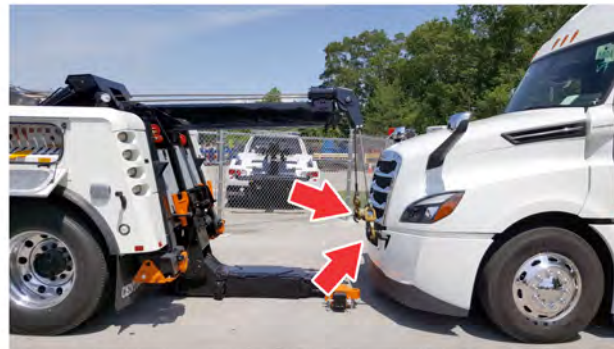
Fig 333, Tow Cables Connected to the Tow Hooks
