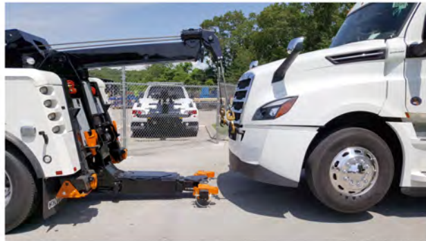
Fig 334, Moving the Stinger and Crossbar Under the Bumper
