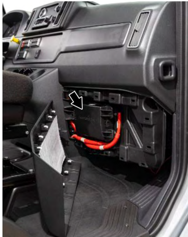
Fig 172, Power Distribution Module (PDMi) Behind Right-Side Dash
