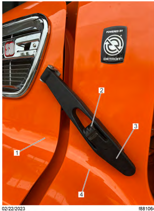
Fig 29, Hood Hold-Down Latch
