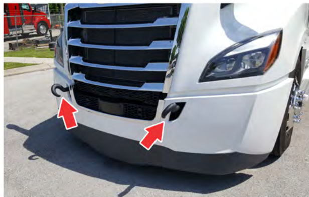
Fig 331, Tow Hooks Installed, Facing Down
