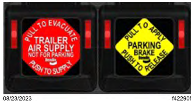
Fig 202, Tractor Parking Brake Set and Trailer Spring Brakes Set
