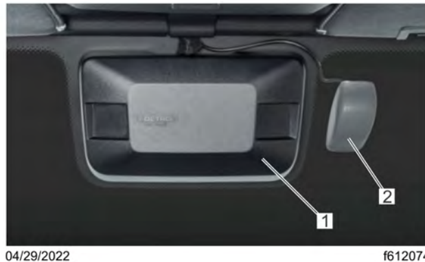
Fig 163, Multipurpose Camera 2 and Bendix Camera Brackets
