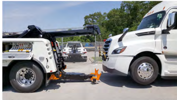
Fig 336, Backing the Tow Truck with Lift Adaptors on the Crossbar
