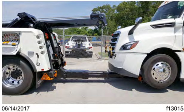
Fig 338, Stinger with Lift Adaptors Under the Axle (tow truck shown)
