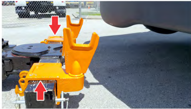
Fig 242, Lift Adaptors Installed on the Crossbar
