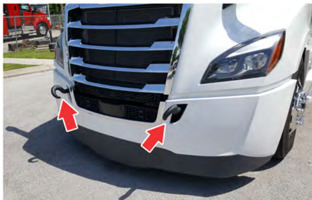
Fig 238, Tow Hooks Installed, Facing Down
