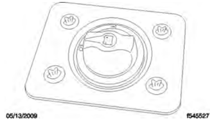
Fig 37, Load Disconnect Switch
