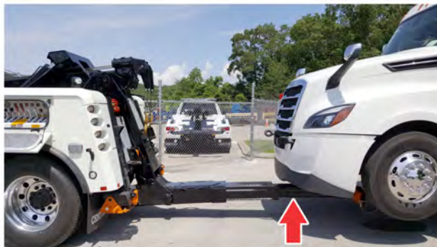
Fig 246, Retracting the Recovery Boom
