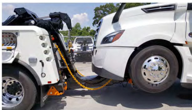
Fig 248, Safety Chains Connected on the Towed Vehicle
