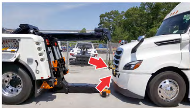
Fig 240, Tow Cables Connected to the Tow Hooks
