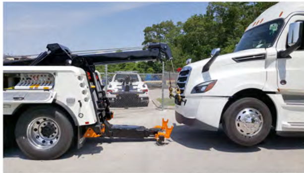
Fig 243, Backing the Tow Truck with Lift Adaptors on the Crossbar
