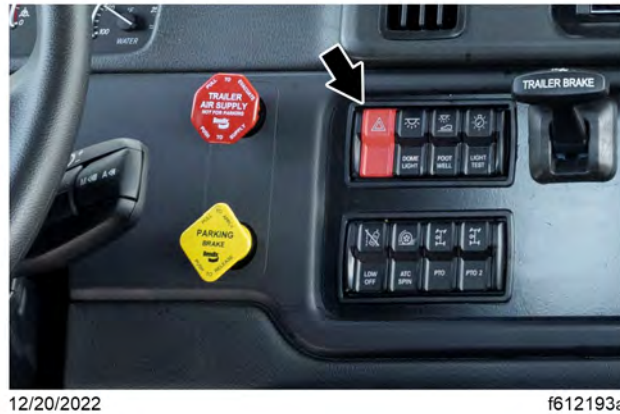
Fig 406, Hazard Warning Switch
