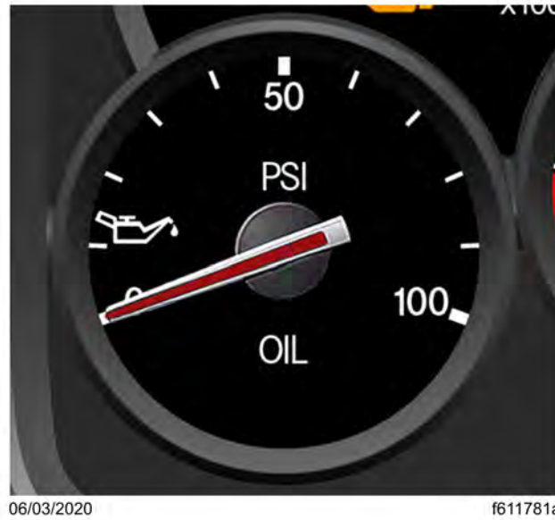
Fig 76, Analog Engine Oil Pressure Gauge - ICUC
