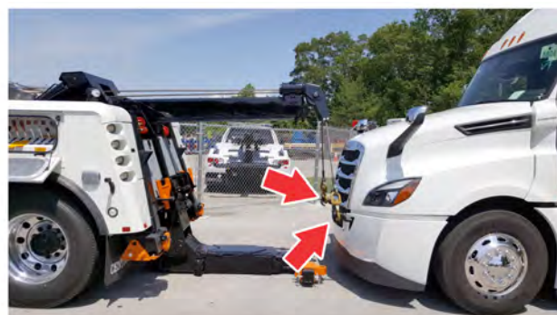
Fig 414, Tow Cables Connected to the Tow Hooks
