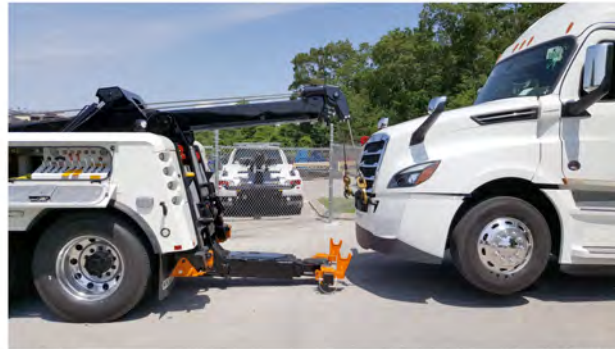
Fig 417, Backing the Tow Truck with Lift Adaptors on the Crossbar
