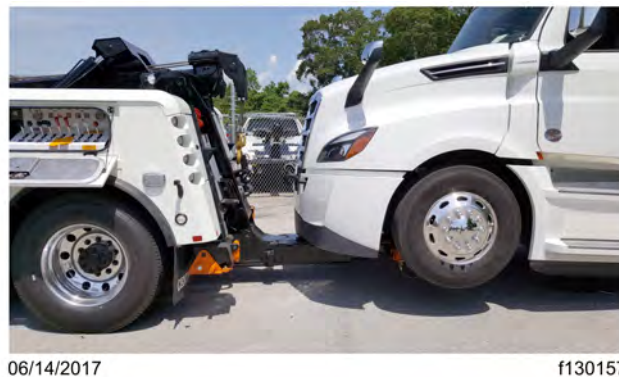
Fig 421, Final Towing Position
