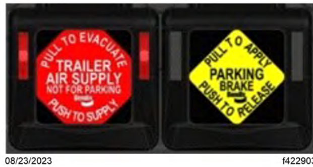
Fig 258, Tractor Parking Brake Released, and Trailer Spring Brakes Set
