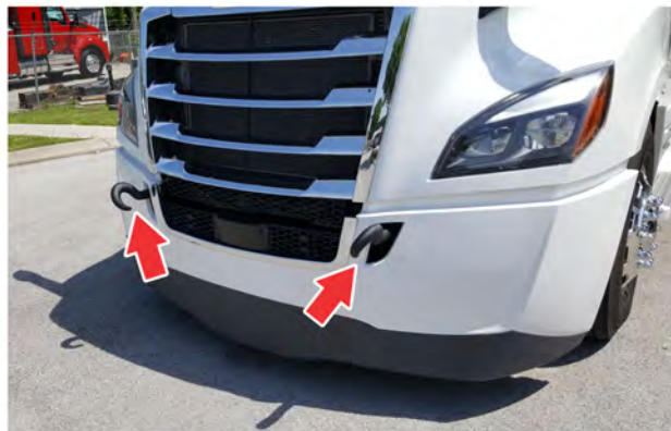
Fig 412, Tow Hooks Installed, Facing Down
