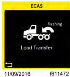
Fig 66, Load Transfer Alert - ICUC
