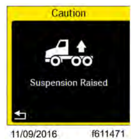
Fig 64, Suspension Raised Alert - ICUC
