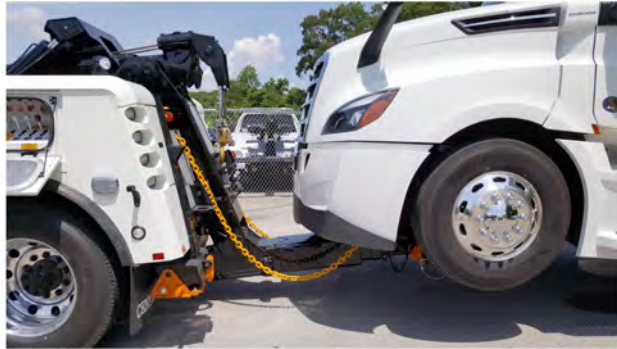
Fig 422, Safety Chains Connected on the Towed Vehicle
