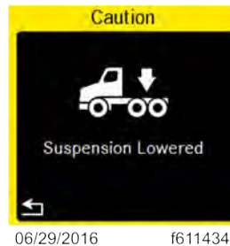
Fig 63, Suspension Lowered Alert - ICUC
