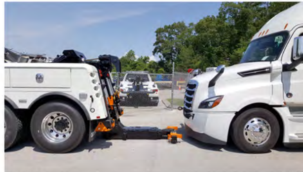
Fig 413, Positioning the Stinger Assembly
