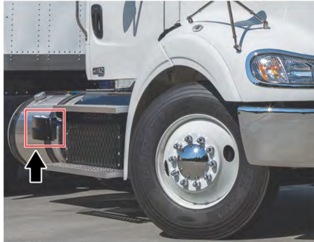
Fig 161, Radar Sensors with Covers
