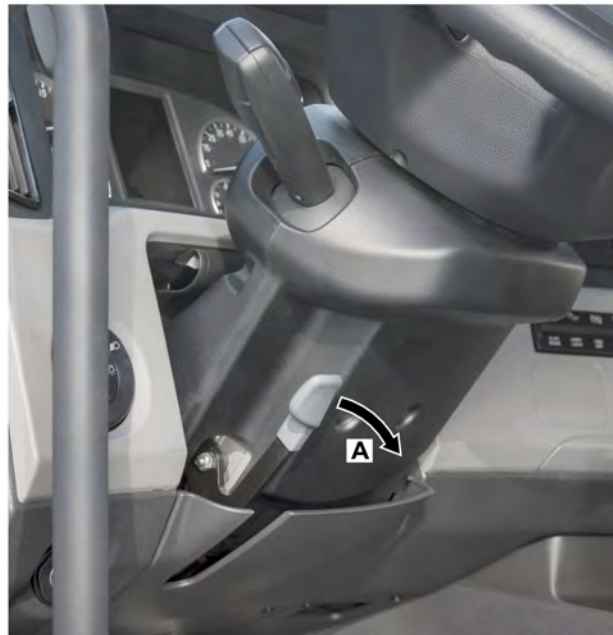
Fig 87, Unlocking the Steering Column
