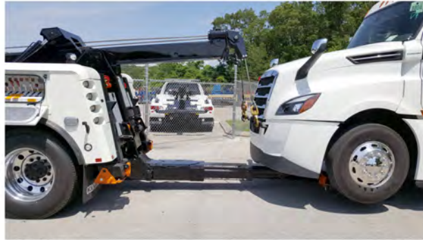
Fig 419, Stinger with Lift Adaptors Under the Axle (tow truck shown)
