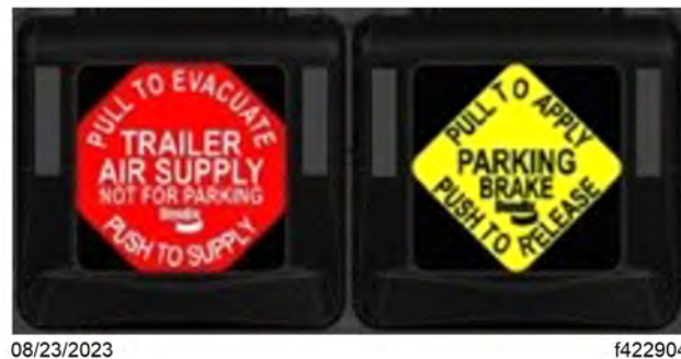
Fig 259, Tractor Parking Brake Released and Trailer Spring Brakes Released
