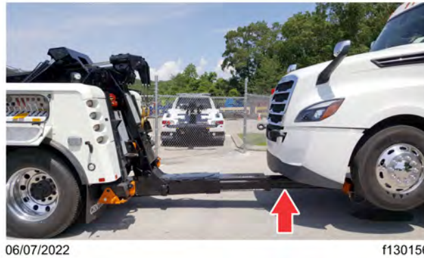
Fig 420, Retracting the Recovery Boom
