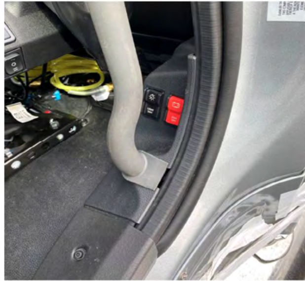
Fig 233, Smart Battery Shutoff Switch
