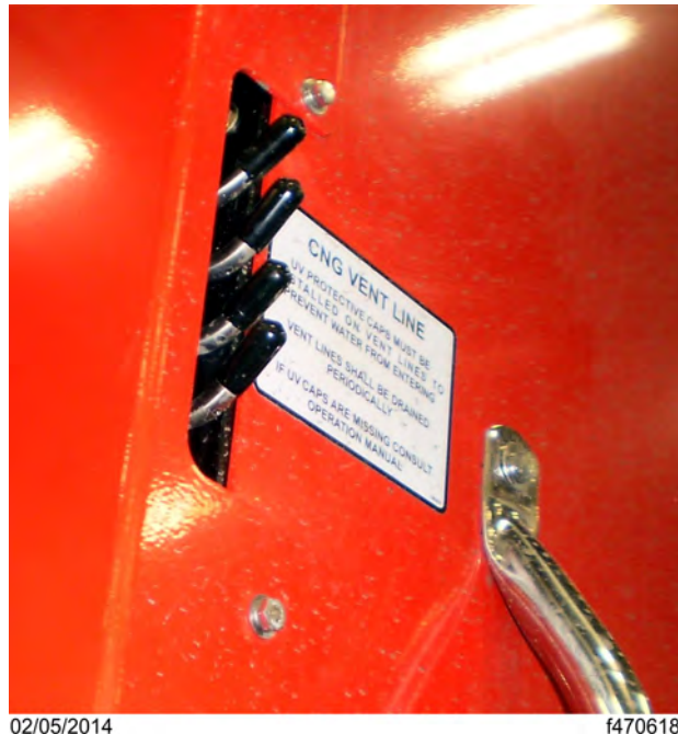
Fig 264, CNG Vent Line Caps
