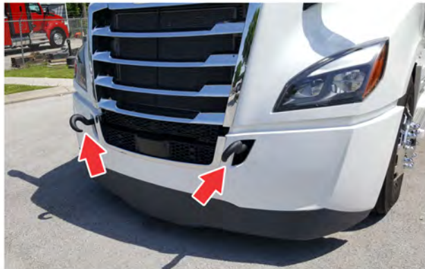
Fig 238, Tow Hooks Installed, Facing Down
