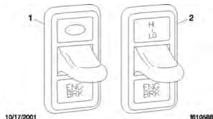
Fig 156, Engine Brake Switches
