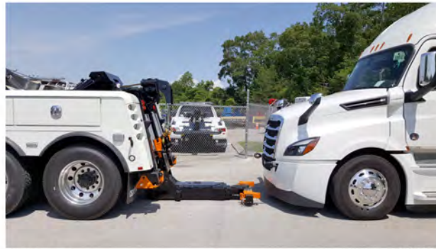
Fig 239, Positioning the Stinger Assembly
