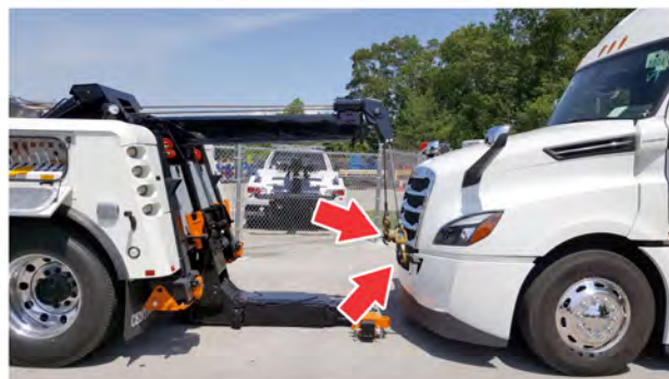
Fig 240, Tow Cables Connected to the Tow Hooks
