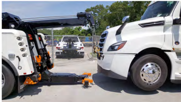
Fig 241, Moving the Stinger and Crossbar Under the Bumper
