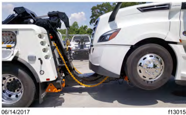
Fig 248, Safety Chains Connected on the Towed Vehicle
