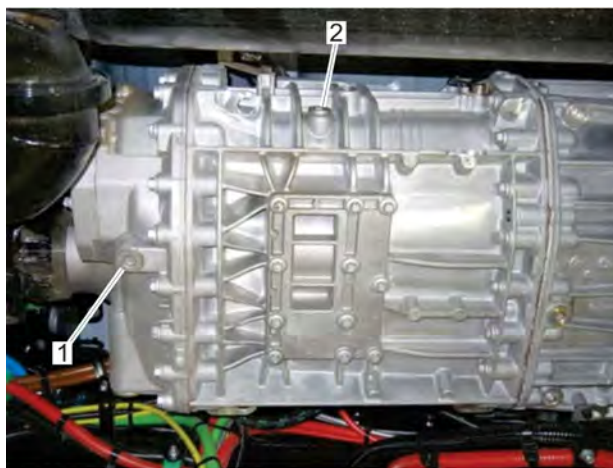
Fig 17, Drain and Fill Plugs, Detroit Automated Transmissions
