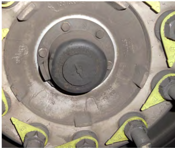
Fig 53, Normal Oil Venting
