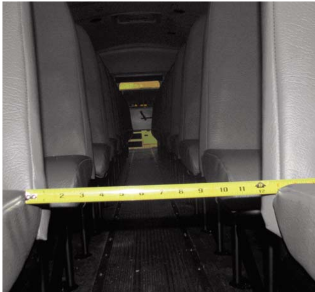
Aisle Width Measurement
