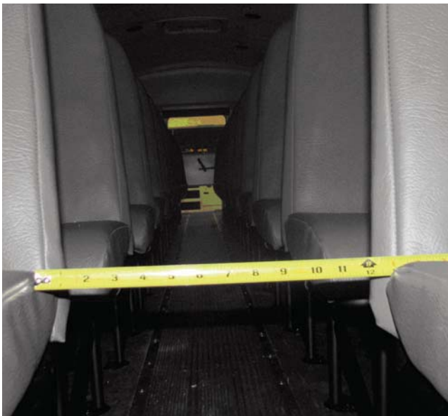
aisle width measurement
