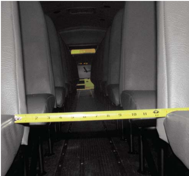
AISLE WIDTH MEASUREMENT
