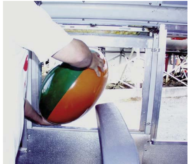
ELLIPSOID GAGE PASSING IN BEHIND OF SEAT
