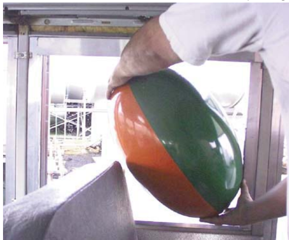
ELLIPSOID GAGE PASSING IN FRONT OF SEAT
