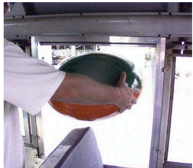
ELLIPSOID GAGE PASSING ABOVE SEAT BACK
